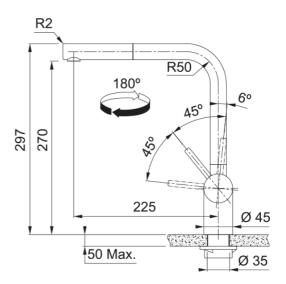
Atlas Neo Pull-Out Nozzle Copper, Overall height 297mm. Side Lever, Ceramic Mechanism, Perlator, useful Pull-Out Nozzle feature.
