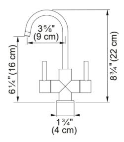
Steel Little Butler® Champagned Gold Two Handle Hot and Cold Water Filtration Faucet. Solid 304 stainless steel construction delivers corrosion resistance inside and out and 360-degree swivel spout provides a full range of motion. For use with Franke undercounter StillPure filtration system. This faucet is not eligible for sale or resale into the State of California due to California's AB100 Legislation.
