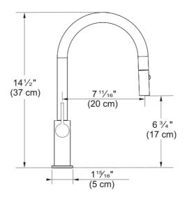
Ambient 14.5-inch Satin Nickel Single Handle Pull-Down Kitchen Prep Faucet. Ambient's solid brass construction ensures long-lasting performance. The ECO cartridge's built-in water saving feature helps conserve water during everyday kitchen tasks. The single handle effortlessly controls water temperature and pressure. ADA compliant.
