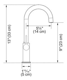
Ambient 13-inch Polished Chrome Single Handle Kitchen Bar Faucet. The ECO cartridge's built-in water saving feature helps conserve water during everyday kitchen tasks. The single handle effortlessly controls water temperature and pressure. ADA compliant.
