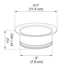
Franke Waste Disposer Flange - SS. Replacement Waste Disposer Flange for Kitchen Sink in Stainless Steel. Stopper included; Hole Size: 3.5-in.
