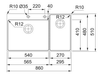
BWX 220-54-27 860X510X200mm, stainless steel brushed, 3 1/2", with waste kit, with tap ledge, workcenter right side, with hidden overflow, with 2 tap holes, in cardboard box
