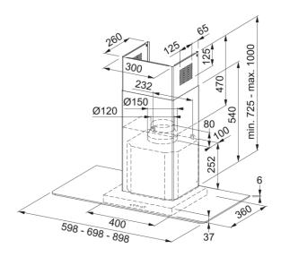
T-Glass Nice 60 FGL 625 XS NP Stainless Steel/Glass, Wall Hood, 60cm wide. Push button controls, 3 speeds plus intensive, 2 x LED Lights. NB Separate Charcoal Filter required if fitting hood in recirculatory mode.
