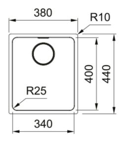
MYTHOS BOWL MYX 110 34 380x440mm, Undermount, Matt Brushed Stainless Steel,  $3\frac{1}{2}$ " Semi-Integrated Waste with Hygienic Overflow. The range features tight bowl radii, a bowl depth of 200mm, and a round flush cover plate giving a smooth base protecting pots and glasses. 50 Year Guarantee on all Franke sinks.
