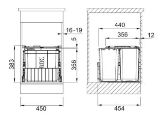
Sorter 300-45 Trio, fits 450mm cabinet.  $1 \times 22$  litre &  $2 \times 10$  litre bins. The roll-out carrier is fully waterproof, simple to dismantle & easy to clean. Separates out domestic waste such as food, cans, plastic and paper. Lid closes over bins to contain any odours. Fits most standard cabinets, mounted on standard cabinet side wall, soft-close mechanism.
