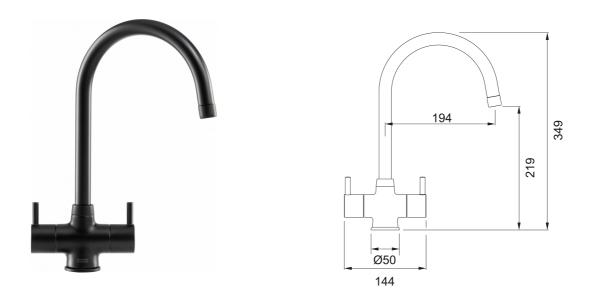
Athena Matt Black finish, Overall height 349mm, Twin Lever, Ceramic Valves, Perlator mixes air into the water to give a champagne- like flow, suitable for low pressure systems.
