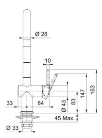
Active J Spout Dual Spray Pull-Down Tap Chrome finish, Overall height 312mm, Side Lever, Ceramic Mechanism. Lever only moves forward, ideal for use with upstands.
