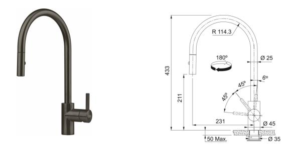
Eos Neo Tap Anthracite, Overall height 433mm, Side Lever, Ceramic Mechanism, useful Pull-Down Spray feature.
