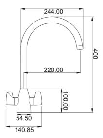
Davos 'J' Tap Decor Steel finish, Overall height 398mm, Twin Lever, Ceramic Valves, suitable for low pressure systems.
