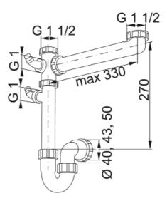
Siphon I Plumbing Kit, for single bowl sinks. Optimises under-sink cabinet space, manifold with incline & air vent for faster water disposal, unique WDU connector, made from rigid grey polypropylene that is highly resistant to burns, dents, chips and stains.
