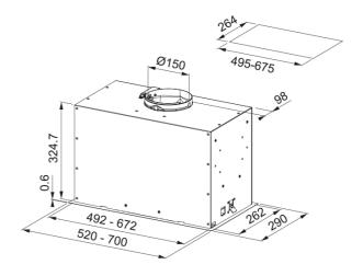
Box EVO 70cm Stainless Steel, FBFE XS A70, Under-Cabinet Hood, Flush mounted. Light temp. 3000K. Push button controls. Blue display colour.
