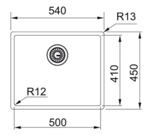
Mythos Masterpeice BXM 210/110-50, Gold PVD coating and nanocoating with F-Inox Technology, Stainless Steel, can be installed as a slim-top, flushmount or undermount, 1 bowl without drainer, 500mm x 410mm, 3 1/2". Includes colour coordinated bottom grid and semi- integrated waste with matching overflow. Additional coloured strainer bowl and rollamat can be bought. 50 Year Guarantee on all Franke sinks. 50 Year Guarantee on all Franke sinks.
