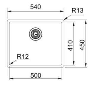
Mythos Masterpeice BXM 210/110-50, Anthracite PVD coating and nanocoating with F-Inox Technology, Stainless Steel, can be installed as a slim-top, flushmount or undermount, 1 bowl without drainer, 500mm x 410mm, 3 1/2". Includes colour coordinated bottom grid and semi-integrated waste with matching overflow. Additional coloured strainer bowl and rollamat can be bought. 50 Year Guarantee on all Franke sinks. 50 Year Guarantee on all Franke sinks. Available early 2025.
