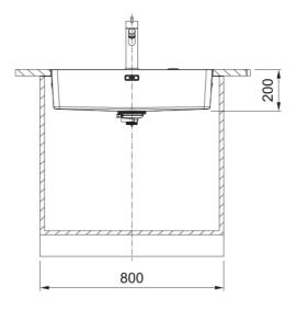
MYTHOS BOWL MYX 210 70 712x412mm, Inset, Seamless 6mm rim to integrate perfectly with the work surface, Brushed Stainless Steel, 3<sup>1</sup>/<sub>2</sub>" Semi-Integrated Waste with Round Flush Waste Cover and Hygienic Overflow. 50 Year Guarantee on all Franke sinks.
