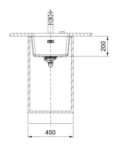
The Franke Maris MRG 110-37 is manufactured from an exceptionally tough material, highly resistant to burns, dents, chips and stains. Pioneered by Franke, it's a unique material with a subtle sheen that is warm to the touch thanks to its close to 80% of quartz sand. The surface is finely textured ensuring high hygiene standards. - Undermount installation. -  $3\frac{1}{2}$ " semi-integrated waste with circular cover-plate and hygienic overflow. - 50 year guarantee on all Franke sinks.
