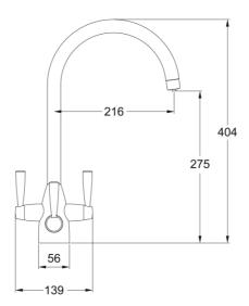
Franke FilterFlow taps deliver hot, cold and filtered water using an advanced ceramic cartridge. <br/>
