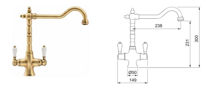
Cotswold Brass tap, Overall height 300mm, Twin lever (new design), Ceramic valves, suitable for low pressure systems.
