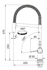
Active Semi-Pro Tap Chrome finish, Overall height 470mm, Pull-Out Spray, Side Lever, Ceramic Mechanism. Lever only moves forward, ideal for use with upstands.
