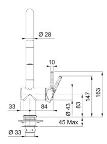
Active J Spout Dual Spray Pull-Down Tap Matt Black finish, Overall height 312mm, Side Lever, Ceramic Mechanism. Lever only moves forward, ideal for use with upstands.
