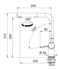
Active L Spout Dual Spray Pull-Out Tap Matt Black finish, Overall height 312mm, Side Lever, Ceramic Mechanism. Lever only moves forward, ideal for use with upstands.
