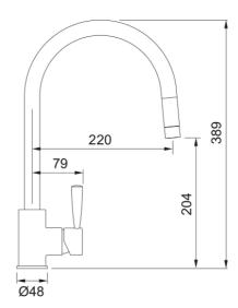
Fuji Pull Out Nozzle Chrome finish, Overall height 390mm, Side Lever, Ceramic Mechanism, Pull-Out Nozzle.
