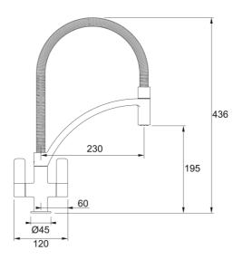
Wave Pull-Out Nozzle Chrome Steel finish tap, Overall height 436mm, pull-out nozzle tap with supporting arm bar, Dual lever control and single-flow swivel spout. Ceramic Disc Valves, Perlator mixes air into the water to give a champagne- like flow. This product is available through our Authorised Internet Partners and National Retailers - please click on the 'Where to Buy' link above. Please quote Product Name and Code as Article Number may differ.
