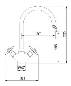
Rotaflow Chrome finish, Overall height 335mm, Twin Handle, Ceramic Valves, Perlator mixes air into the water to give a champagne- like flow, suitable for low pressure systems.
