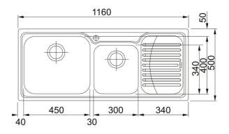
GALASSIA GAX 621 1160x500mm, Inset, Right Hand Drainer, Silk Stainless Steel,  $3\frac{1}{2}$ " Wastes with Slotted Overflow, 1 tap hole. Model will not accommodate taps with a base over 55mm. 50 Year Guarantee on all Franke sinks.
