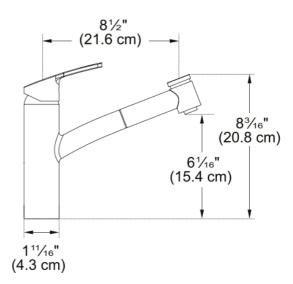
8.8-in Single Handle 1-Hole Polished Chrome Pull-Out Kitchen Faucet. Our top-quality Smart faucets are equipped with a long extendable nozzle enabling you to fill large pots quickly and giving you all the freedom to work in and around your sink. They come with a Franke ceramic disk cartridge to guarantee excellent, long- lasting, smooth water flow. ADA Compliant. This model replaces the FFPS3600 Faucet
