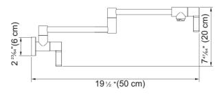
Ambient 5.2-in Two Handle Polished Chrome Wall Mounted Pot Filler. Two handle design offers control at the point of use and wall and the 180-degree spout swivel range provides ample reach and rotation for filling large pots on stovetops.
