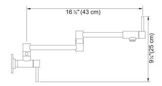
Two Handle Stainless Steel Wall Mounted Pot Filler. Solid 304 stainless steel construction that delivers corrosion resistance inside and out. Two handles that offer control at the point of use and wall and the 180-degree spout swivel range provides ample reach and rotation for filling large pots on stovetops. ADA Compliant. This model replaces the Steel PF3450 pot filler.
