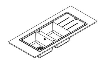
7 Fasten Sink Clips to underside of worktop. Leave for 12-24 hours for sealant to set before starting on the plumbing.
