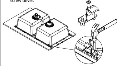
5 Put a bead of sealant around the top edge of cutout to seal the Sink/Basin to the worktop and to stop water from leaking into your cupboard.
