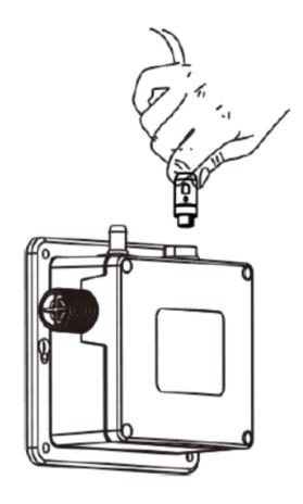
Connect water outlet hose from spout to control box. Secure with clamp.
