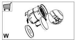
The grease filters must be cleaned every 2 months of operation or more frequently in case of very intense use and can be washed in a dishwasher (Z).
