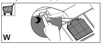
The grease filters must be cleaned every 2 months of operation or more frequently in case of very intense use and can be washed in a dishwasher (Z).
