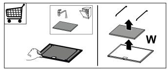
The grease filters must be cleaned every 2 months of operation, or more frequently in the case of particularly intensive use. They can be washed in a dishwasher (Z).
