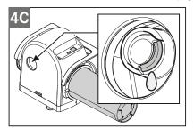
CAUTION: If no expansion water runs off during heating, switch off the power supply immediately and open the hot water tap to relieve the water pressure. Refer to the troubleshooting guide.
