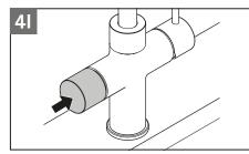
Filling mode short: Press briefly 2x. Stops automatically. Deactivate; press briefly 1x (fig. 4J).
