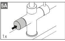
► Hold depressed for 10 seconds, as LED lights up again (fig. **5B**).
