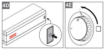
When the boiler is switched on, the temperature of the water is automatically held constant so that boiling water is available at any time of the day. In order to prevent the temperature of the boiler being unnecessarily held constant, you can use the energysaving ECO mode. After activation, ECO mode comes into operation every day at the same time. The duration of ECO mode is 6 hours and the LED should light up green during this time.
