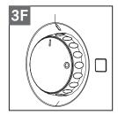
The status of the boiler is signalled by a lamp alongside the rotary knob. When the water is being heated, this lamp lights up red.
