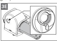
WARNING: If, during heating, no expansion water has escaped after 10 minutes: Switch off the power supply immediately and turn on the boiling water tap to relieve the water pressure.
