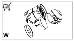
The grease filters must be cleaned every 2 months of operation or more frequently in case of very intense use and can be washed in a dishwasher (Z).
