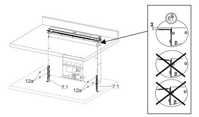
• With the aid of a spirit level, set the Hood Canopy level vertically and fix it to the Lower Surface using 2 screws 12c provided.
