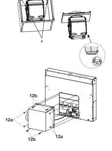
Connect the Electric cables that come out of the lower right hand part of the Hood Canopy to the Connectors on the Electric unit.
