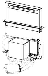
Marning..: Do not install the product in such a way that the wiring box is in contact with the floor.
