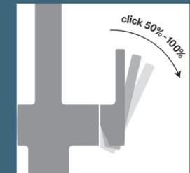
Sufficient water pressure at just 50% open
