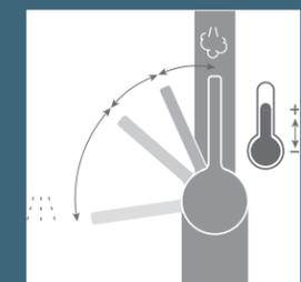
Remove the lever and turn the ring nut inside to limit the flow temperature\*
