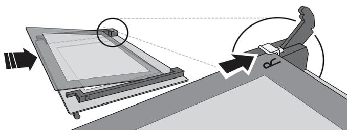
4. Refit the upper edge: a click will indicate correct positioning. Make sure the seal is secure before refitting the door.
